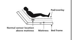
BED: Place sensor pad under the sheets in the hip area. Run sensor pad cord under mattress towards M210. Plug sensor pad into the M210.
